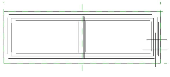
In Revit start creating an extrusion (Ribbon: Create  $\rightarrow$  Group: Forms  $\rightarrow$  Extrusion  $\square$ ). Revit switches to the sketch editing mode.
