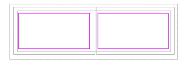
Finish the sketch by confirming the green checkmark ✓ and switch to the "Re. Level" view. You can see the new extrusion object connected to our "Mounting depth" reference plane. Now we can adjust the extrusion depth as well as the extrusion direction.
