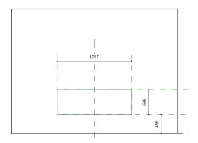
Next we want to adapt the already existing family parameters to the exact dimensions. In Revit open the "Family Types" Dialog  $\stackrel{\square}{=}$  (Ribbon: Modify  $\rightarrow$  Group: Properties) and change the values for "height", "width" and "sill height" according to the exact sizes:
