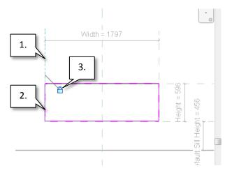
Repeat the process with the other tree edges and finish the sketch mode. Now we can "flex" the parameters for "height" and "sill height" and the opening will adjust correctly (don't forget to go back to the previous values after flexing, otherwise our project coordinates are no longer correct).
