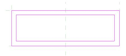
Finish the extrusion by confirming the green checkmark  $\checkmark$ .
