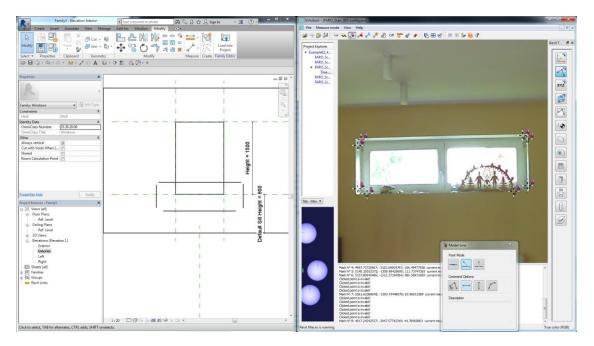
Now we have the "skeleton" for the new window opening. Select the opening rectangle in Revit (use the [tab] key to select the right object!). The green context Ribbon "Modify | Opening cut" appears. Select "Edit Sketch" in the Group: Opening.
