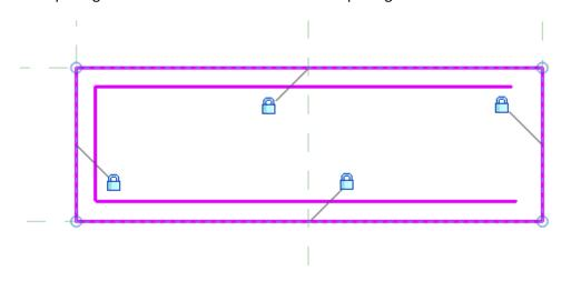
Choose the "Trim/Extend to Corner"  $\stackrel{\text{def}}{\rightarrow}$  tool (Ribbon: Modify|Opening  $\rightarrow$  Create Extrusion  $\rightarrow$  Group: Modify) and click the inner three lines one after the other to trim the corners.
