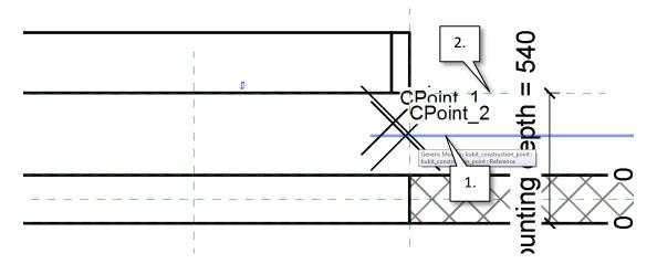
With the align command still active click on the reference at the second construction point (CPoint\_1) and afterwards on the upper edge of the extrusion form (use the [Tab] key to select the right face).
