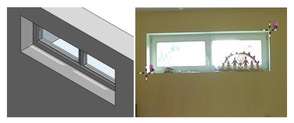
If the orientation of the window is in the wrong direction (interior and exteriour side), you can flip the instance in the "Level 1" view by selecting the window and clicking the symbol with the two blue arrows.
