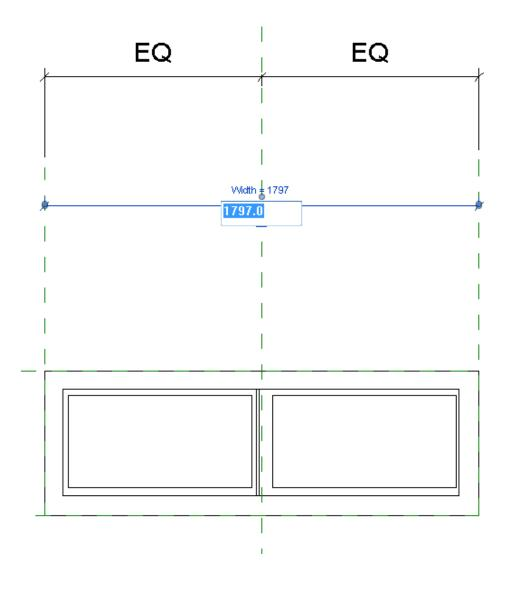
Let's complete the family with an object for the glass pane. Open the "Interior" view in Revit and
