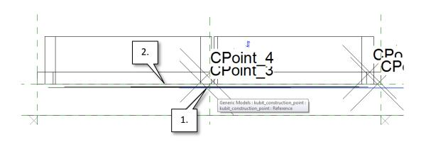
With the align command still active click on the reference at the second construction point (CPoint\_4) and afterwards on the upper edge of the extrusion form (use the [Tab] key to select the right face).
