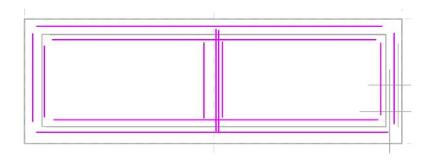
With the "Split Element" is tool (Ribbon: Modify|Create Extrusion  $\rightarrow$  Group: Modify  $\rightarrow$  Split Element ) you can cut the four horizontal lines near the midpoint. Now it is possible to complete the sketch with the "Trim/Extend to Corner" it tool (Ribbon: Modify|Opening  $\rightarrow$  Create Extrusion  $\rightarrow$  Group: Modify).
