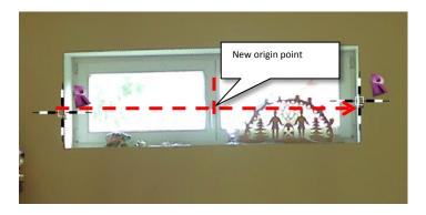
Now choose the "z height" option and click a point a few centimeters below the window. It need not be exact because the sill height will be parameterized later:
