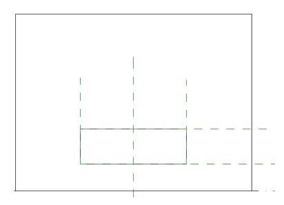
Next step is adding new dimension for the family parameters between the reference planes. Choose the "Aligned" dimension  $\checkmark$  tool (Ribbon: Annotate  $\rightarrow$  Group: Dimension). Click on the first plane then on the second one and after that finish the command by clicking next to the second plane. Create three dimensions for "height", "width" and "sill height":
